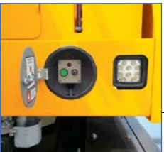
▲ Bridge device switch
