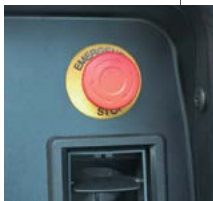
▲ Emergency engine stop switch (for crane operation)
